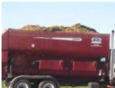
An example of a load that is too full and will not mix properly
